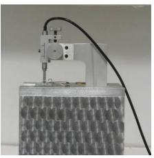
*Elastic recovery measuring system,* PC-controlled, with load cell (K5) and A/D converter (*Pico*).
