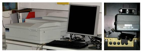
**RamSpec Raman spectrometer/BaySpec** (portable fiber-optic based Raman spectrometer with microscope attachment, and probes-ø: 6mm and 1.2 mm- for in vivo skin and tooth analysis. The 6 mm probe can be connected to the Nikon Eclipse ME 600 microscope for microanalysis).
