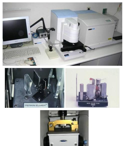
*Lambda 35 UV-Vis spectrometer/ PerkinElmer* (with a 50 mm integrated sphere for total transmittance and diffuse reflectance measurements, including colorimetry software)
