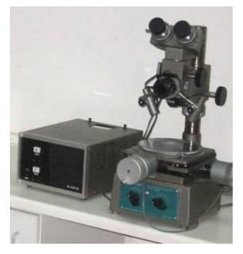
*M80/Leica* (Transmission/reflection stereomicroscope, with uniaxial, coaxial and lateral LED illumination and *Leica DFC295* digital camera).
