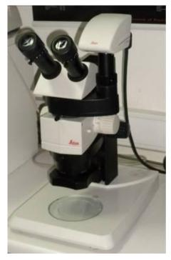
*Elvar/Leitz* (Stereomicroscope, with *Leica CLS 100 X* uniaxial and lateral fiberoptic illumination and *Coolpix 990/Nikon* digital camera).
