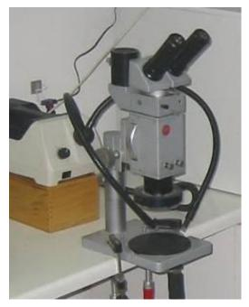
*Micro-Scopeman/Moritex* (Portable video-microscope, with uniaxial fiberoptic illumination, contact and non-contact lenses).
