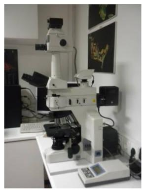
STM/ Olympus (Transmission/reflection digital micro-measuring microscope).
